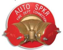
For both inlets and outlets, the escutcheon provided with each fire department connection shall be of aluminum construction and have a red background with white letters identifying the service design.
