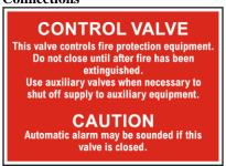
The caution sign shall be worded as follows: This valve controls fire protection equipment. Do not close until after fire has been extinguished. Use auxiliary valves when necessary to shut off supply to auxiliary equipment. CAUTION: Automatic alarm can be sounded if this valve is closed
